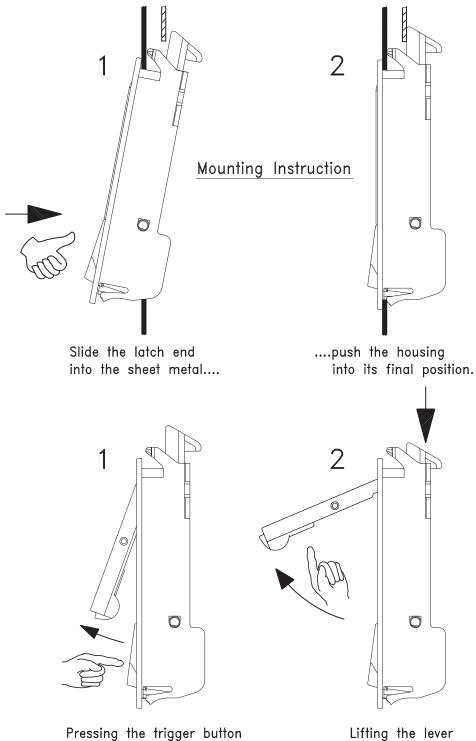
Pressing the trigger button releases the lever and jumps up. The slam latch stays closed. Lifting the lever opens the latch.
