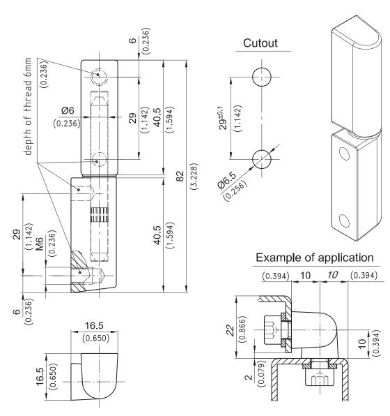
Part No. See Page Corner hinge 224-9008 Screws M6 are not included. Tool-less installation version 04.23
