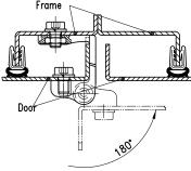
180° if hinges are installed on the left OR on the right. Frame
