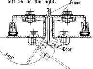
146° if hinges are installed on the left AND on the right.
