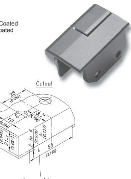
door-notch \*Only notch in case you prefer a narrow gap (1-2mm) between door and frame.
