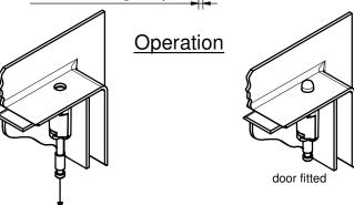
pull the spring-loaded pin for installation and removal of the door
